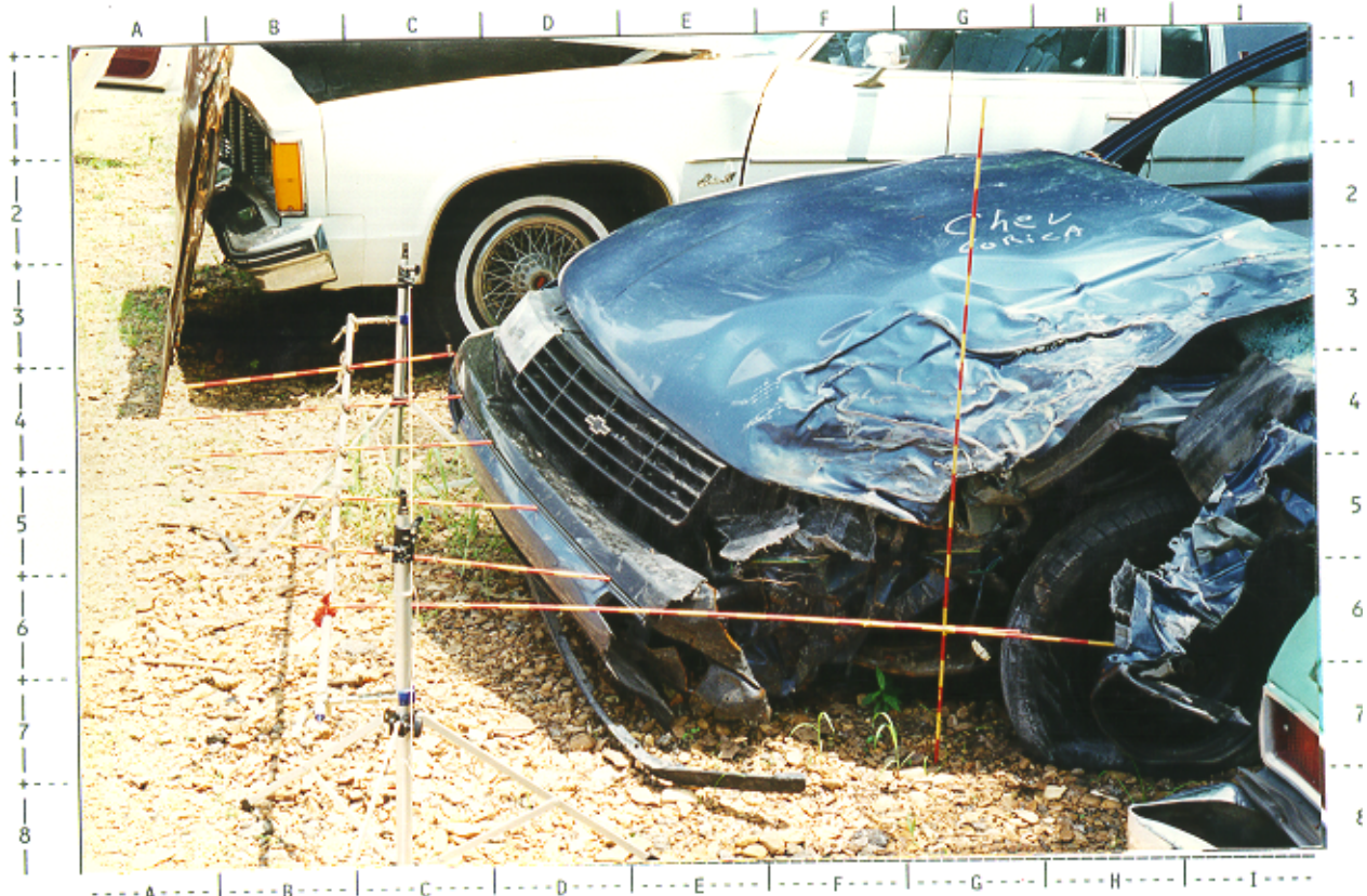
# 34 -- Front reference line viewed from left showing frontal damage to 1991 Chevrolet Corsica; NOTE: maximum crush and vertical rod
